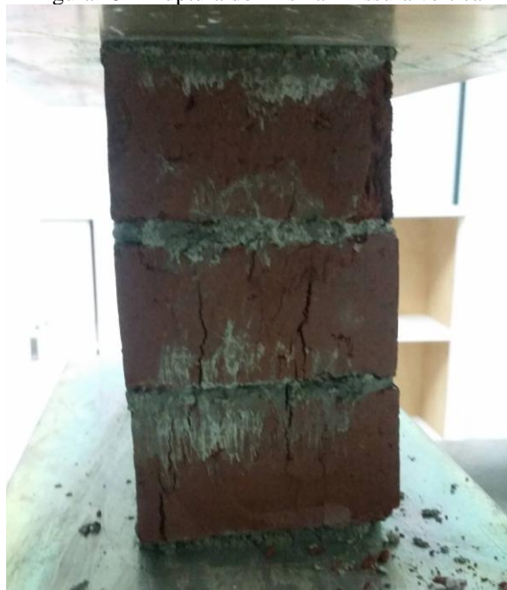
Figura 45 – Ruptura do Prisma – fissura vertical
