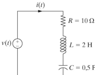
$$v(t) = iR + L \frac{di(t)}{dt} + \frac{1}{C} \int_0^t i(t) dt$$
